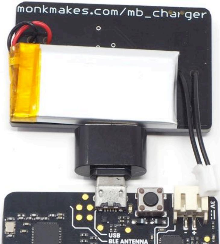
If the USB plug won't fit into the micro:bit's USB socket make sure that the black USB adaptor hasn't been put onto the Charger for micro:bit the wrong way around.
