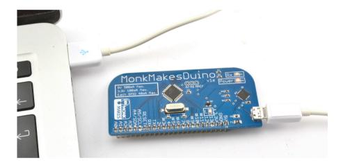
As soon as you connect the MonkMakesDuino, the PWR LED should light and the 'L' LED start to slowly blink. This means that the MonkMakesDuino works and is drawing power from the USB port. If you have a Windows computer ignore the 'Found New Hardware' wizard and disconnect the MonkMakesDuino before the next step, which is to install USB drivers so that you can communicate with the MonkMakesDuino and program it.
