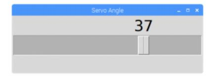
When you run the program, a window will open with a slider. Move the slider left and right and the servo should follow.
