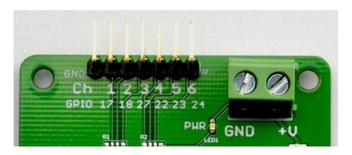
Looking at the picture above, the left most pin is GND and should be connected to a GND pin on the Raspberry Pi. The next pin along (control pin 1) should be connected to GPIO17 on the Raspberry Pi, control pin 2 on the ServoSix to GPIO18 and so on.
