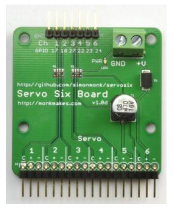
GND on the ServoSix board. For each servo (up to six) that you want to control, you also need a female to female jumper wire connecting the control pin for that servo on the ServoSix board to one of the GPIO pins on the Raspberry Pi.
