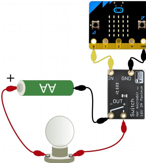
Note that unlike the similar product the MonkMakes *Relay for micro:bit*, the Switch for micro:bit must be connected the right way around with the more positive voltage at the + connection. The switch uses a type of transistor called an n-channel MOSFET and this type of switching is called low-side switching because when the MOSFET turns on, the load is connected to GND (the low side).
