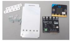
**Step 1.** Start by finding the acrylic piece marked with an **A**, the two spacers marked with a **D**, the Servo for micro:bit board and your micro:bit. You will also need five of the steel nuts and bolts.
