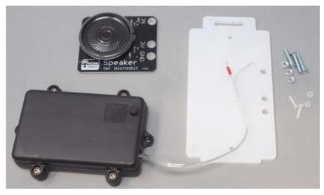
**Step 6.** Start by finding the acrylic piece marked with an **B**, the battery box, the MonkMakes Speaker for micro:bit, 3 pairs of steel nuts and bolts and two sets of plastic nuts and bolts.
