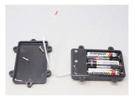
**Step 5.** Unscrew the four screws that hold the battery box together and remove the lid. Insert three AA batteries into the holder making sure that each battery is the correct way around. Then reassemble the battery box.
