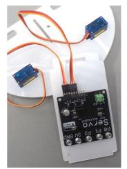
(counter-clockwise) the two screws on the green terminal block on the Servo for micro:bit board. Undo them as far as they will go.
