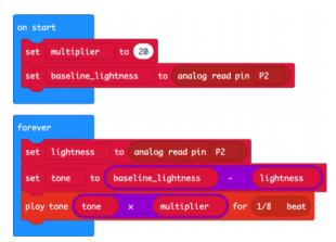
The variable *multiplier* is initially set to 20. This is used to increase the value of the calculated light level to an audible frequency. So, if when you wave your hand in front of the light sensor, all you hear are clicks, then try increasing this value. On the other hand, if, as you move your hand closer to the light sensor, the pitch of the sound rises too high to be audible, try decreasing the value of *multiplier* to 10.
