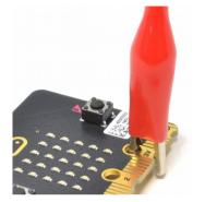
Connecting the alligator clips like this prevents any accidental connections between the large connectors with the holes in and the much smaller connectors (gold lines in the photo above)
