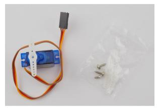
The smallest of the screws in the servomotor's bag is intended to secure the servo arm into place, but you don't need to use it, as the arm should stay in place without it.
